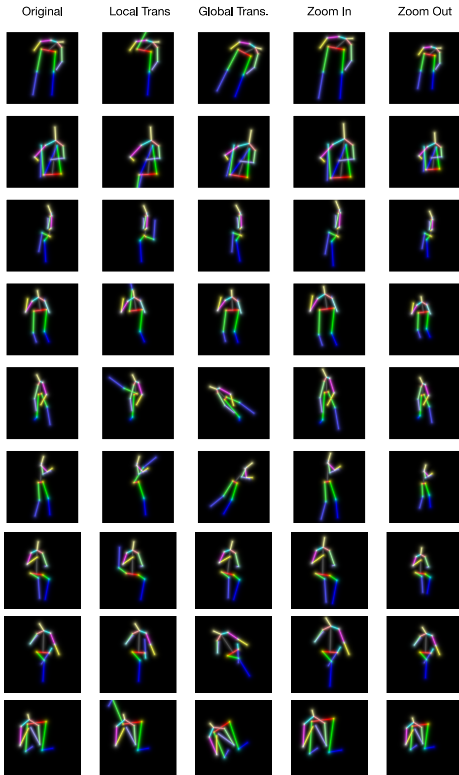
Figure 10: Illustration of augmentations. All of them generate skeleton images that less frequently appear in source targets.
